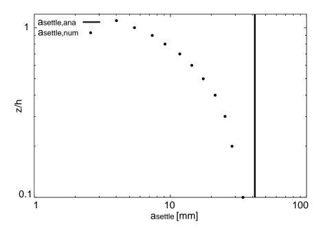
Figure 9: The maximum dust size  $a_{\text{settle}}$  at each height. The points show the numerical results. The solid line shows the analytical results.
