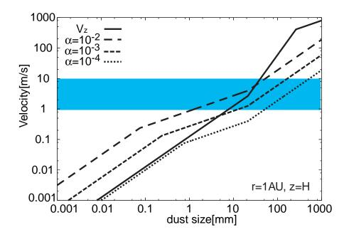
Figure 5: The velocity of the turbulent eddy. We show the relative velocity  $V_{\rm rel,t}$  and  $V_z$  at r=1 AU, z=H. The solid line is the settling velocity  $V_z$ . The long dashed line, the short dashed line and the dotted line are  $V_{\rm rel,t}$  for  $\alpha=10^{-2},10^{-3}$  and  $10^{-4}$ , respectively. The hatched region shows the critical velocity (1-10 m/s).
