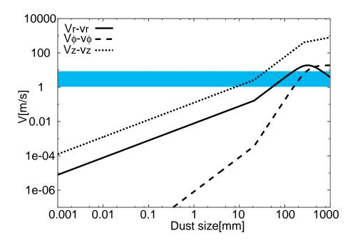
Figure 2: The size dependence of the relative velocity between dust and gas at r = 1 AU, z = H. The solid, the dashed and the dotted lines are  $V_r - v_r, V_\phi - v_\phi$  and  $V_z - v_z$ , respectively. The hatched region shows the critical velocity  $V_{\text{frag}}$ .
