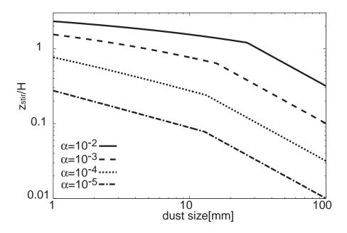
Figure 7: The height to where dust grains are stirred up at r=1 AU. The solid line, the dashed line, the dotted line and the dash-dotted line are  $z_{\rm stir}$  for  $\alpha=10^{-2},10^{-3},10^{-4},10^{-5}$ , respectively.
